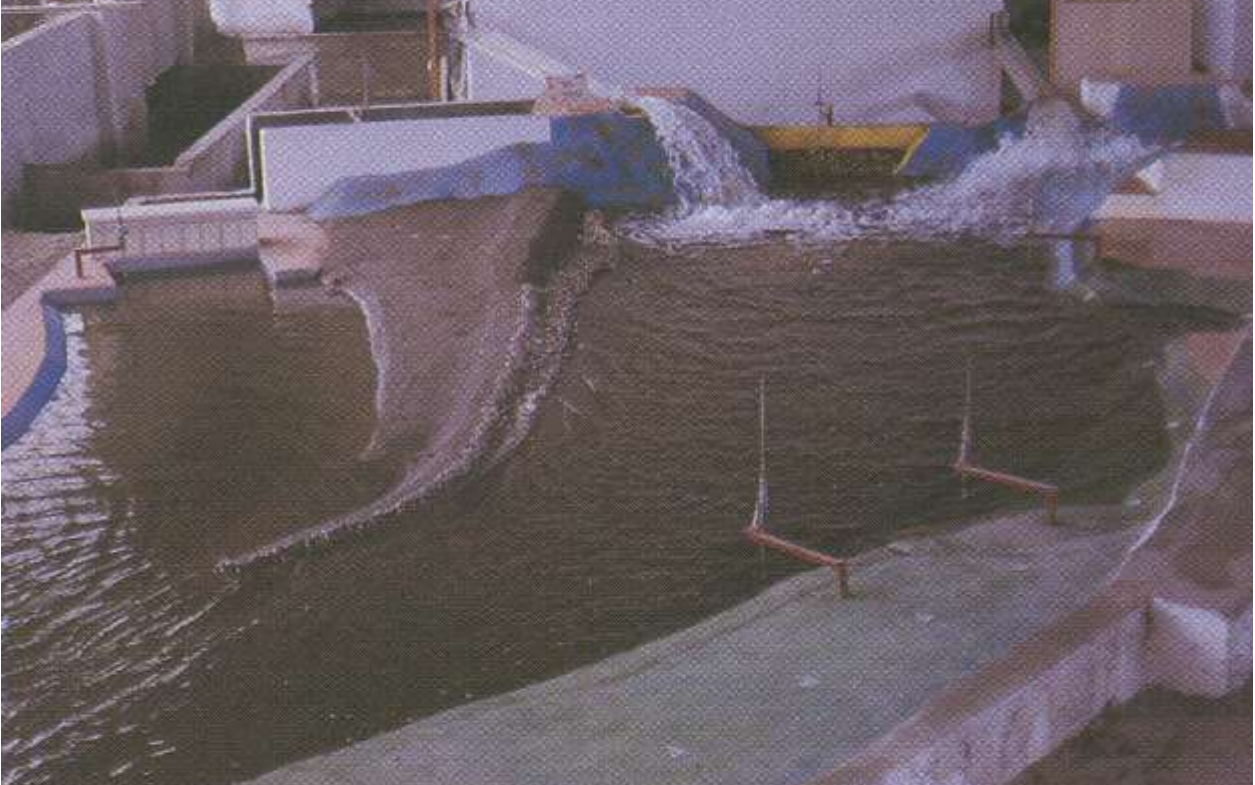
Physical Model of dam spillways, HEPP Koman
