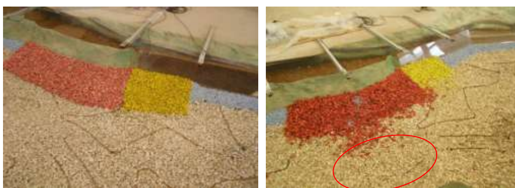
Figure 12: Left bank slope protection zones considering heavy riprap (red), intermediate riprap (yellow) light riprap (blue). Situation before testing (left) and after Test H (Right)
